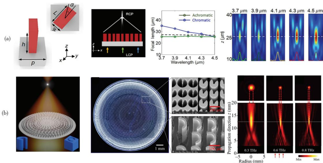
**Fig.6** Continuous achromatic metalenses at other range. (a) Metalens made of Si nanobricks to realize an unchanged focal length in mid-infrared from 3.7 to 4.5  $\mu\text{m}$ <sup>[72]</sup> (Reprinted with permission from Ref.[72]. Copyright 2019, American Physical Society); (b) Broadband achromatic metalens in terahertz regime from 0.3 to 0.8 THz<sup>[73]</sup> (Reprinted with permission from Ref.[73]. Copyright 2019, Science China Press)
