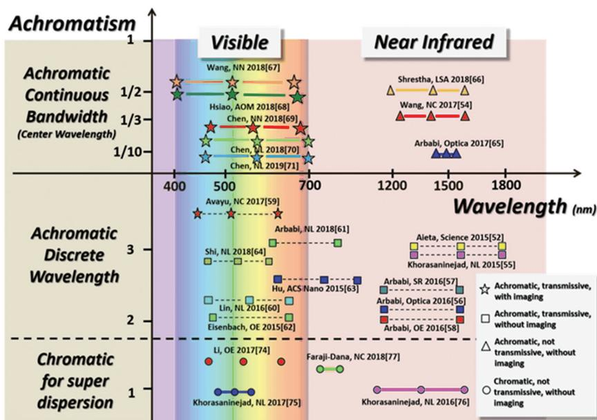
Fig.8 State-of-the-art achromatic metalenses or super dispersion
